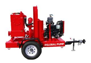
Global Pump\* Standard Centrifugal Wellpoint pumps are specifically designed to effectively handle the arduous requirements of wellpoint and underdrain dewatering systems where intermittent water flow and large amounts of air are encountered. The dual diaphragm priming system generates up to 100CFM without the need for an oil-cooled vacuum pump.
